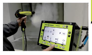
The **Inogun M** is designed to provide the best quality powder application because it is well-balanced, supplied
