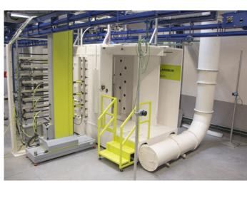
Reduced air speeds in the automatic application area to maximize application yield, and high air speeds at the entry/exit silhouettes to limit powder outflow.
